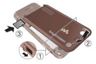
Open the cover and insert the memory card with the gold-coloured contacts facing down.
