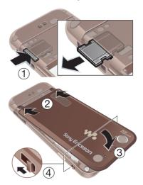
Open the cover and press the edge of the memory card to release and remove it.
