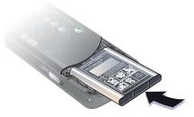
3 Insert the battery with the label side up and the connectors facing each other.
