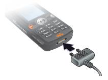
1 Connect the charger to the phone. The symbol on the charger plug must face upwards.
