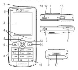
Music button Screen Selection keys Activity menu key Back key Light Memory Stick Duo slot 9 Microphone 10 Power on/off button 11 Ear speaker 12 Camera zoom, volume buttons and picture zoom 13 Navigation key 14 Clear key 15 Camera button 16 (#¬₮) Silent kev
