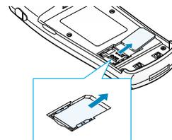
4. Place the battery so that the tabs on the end align with the slot at the bottom of the phone.
